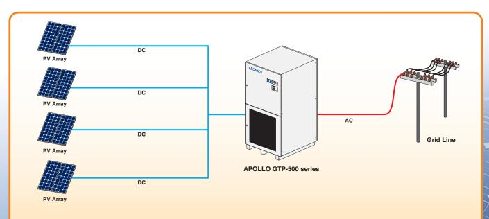
The APOLLO GTP-500 Series is high performance three phase grid connected central inverter that integrated with PV maximum power point trackers (MPPT) to extract maximum power generated from the PV arrays, and also system protection during failure of utility grid power supply. The APOLLO GTP-500 series inverter is suitable for medium to large scale grid connected solar power system.
